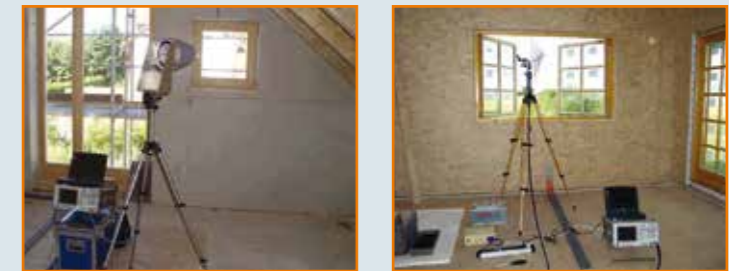
After-check within a house subsequent to shielding
